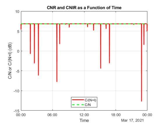
The downward spikes indicate interference. The more severe spikes are caused when simultaneous interference from multiple satellites exists or when an interfering satellite overflies the ground station.
