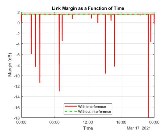
Any time the link margin is greater than or equal to 0 dB, the downlink is closed. With interference, times exist when the link margin dips below 0 dB and at these times the downlink is broken because of interference.
