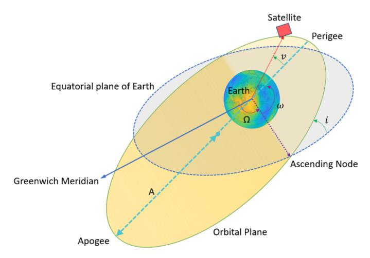
Per Kepler's second law of planetary motion, the angular velocity (rate of change of true anomaly) is different at different locations in the orbit. You can define the mean anomaly, whose rate of change is constant over the entire orbit of the satellite. In GPS ephemeris parameters, rather than specifying true anomaly, mean anomaly is specified (from which true anomaly can be found). IS-GPS-200L Table 20-IV [1] on page 2-0 specifies the algorithms that relate mean anomaly and true anomaly.
