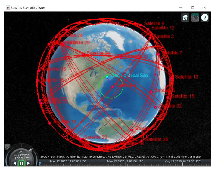
The presence of the geographical site inside the contour is a visual confirmation that it is inside the field of view of the camera onboard Satellite 4.
