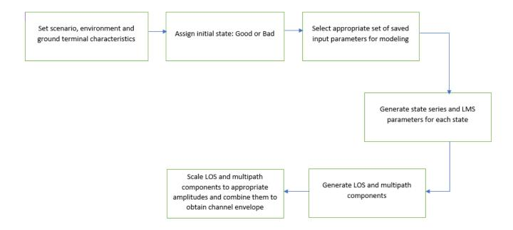
In addition to the environment and carrier frequency defined for this example, the modeling of the channel is done by setting up the scenario. This requires defining the following parameters:
