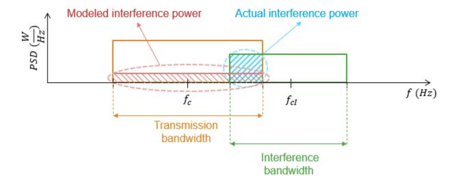
This example assumes that the transmission (or signal) bandwidth of the geosynchronous satellite is 30 MHz and that the bandwidth of the interfering signal is 20 MHz.
