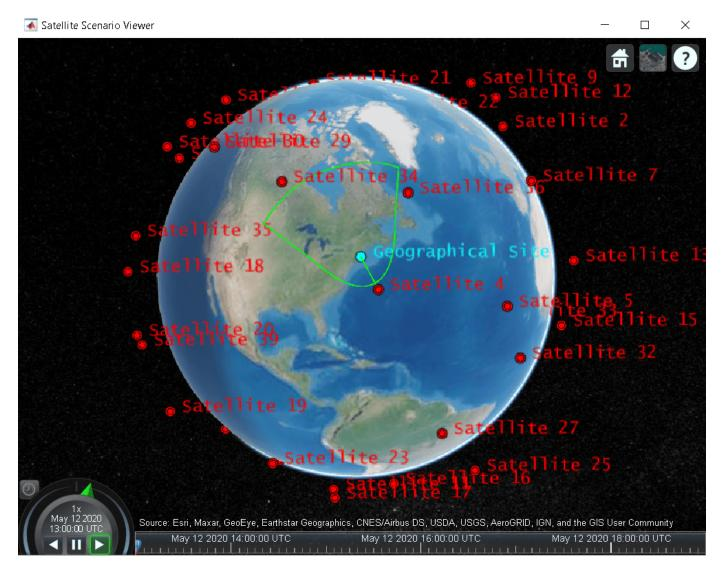
The field of view contour is no longer circular because the camera is not pointing straight down anymore as it is tracking the geographical site.
