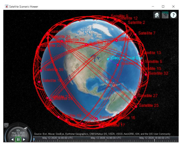
The viewer may be used as a visual confirmation that the scenario has been set up correctly. The violet line indicates that the camera on Satellite 4 and the geographical site have access to one another. This means that the geographical site is inside the camera's field of view and the camera's elevation angle with respect to the site is greater than or equal to 30 degrees. For the purposes of this scenario, this means that the camera can successfully photograph the site.
