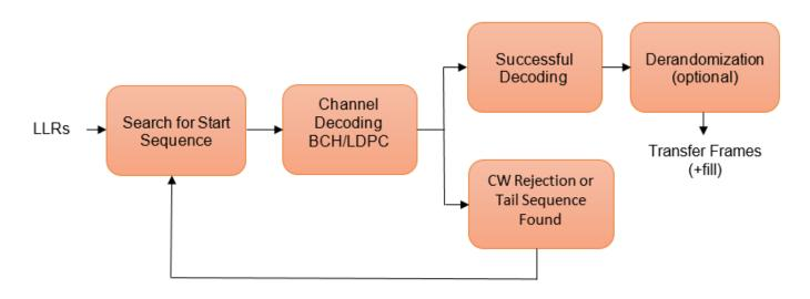
Search for start sequence: When the channel coding is BCH, the incoming bit stream is searched bit by bit for the start sequence pattern. When the channel coding is LDPC, the incoming soft
