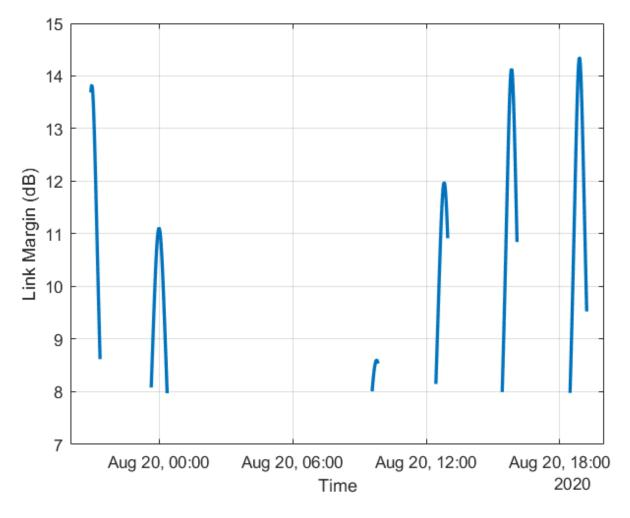
The gaps in the plot imply that the link was broken before reaching the final node in the link, or the line of sight between final node and the node before it, that is, Satellite 2, was broken. At all other times, the link margin is positive. This implies that Satellite 2 Transmitter power and Ground Station 2 Receiver sensitivity are always sufficient. It also implies that the margin is positive at all other hops of the link.
