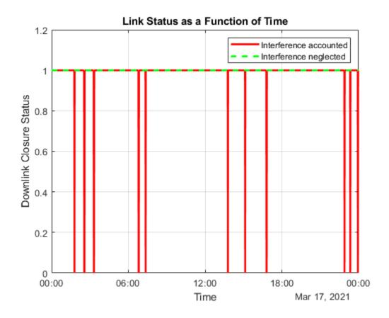
The plot shows times exist when the downlink cannot be closed because of interference. The interference is particularly severe when at least one satellite flies overhead. For instance, the plot shows that the downlink is broken at times such as 1:47 AM, 2:33 AM, and 3:26 AM. Set the CurrentTime property of the Satellite Scenario Viewer to these times to confirm that an interfering satellite overflying the ground station exists.
