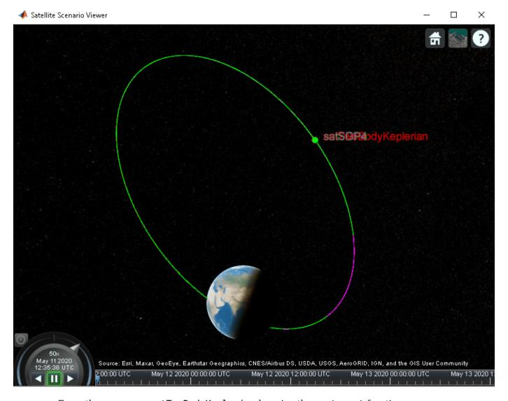
Focus the camera on satTwoBodyKeplerian by using the camtarget function.
