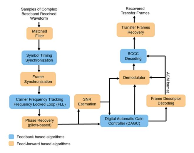
In the receiver chain, frequency locked loop (FLL) uses the frame marker (FM) that is available in the physical layer (PL) header. The phase recovery module uses the pilot fields to recover the phase. Because the phase recovery algorithm is pilots-based, you must enable the pilot fields for the example to work. The phase recovery module can tolerate some amount of residual CFO that is left after the FLL operation.
