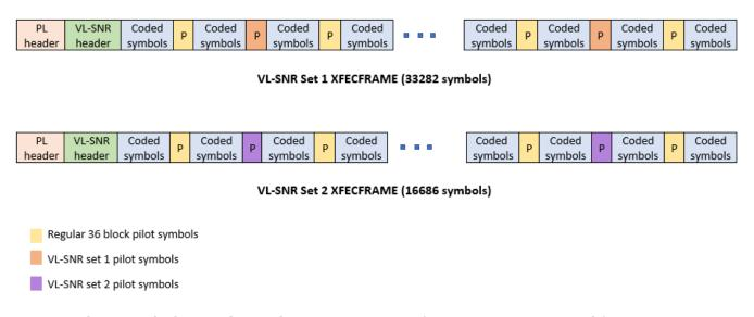
This example designs the synchronization aspects of a DVB-S2X receiver used for VL-SNR applications. The example supports all the nine MODCODs defined by the standard.
